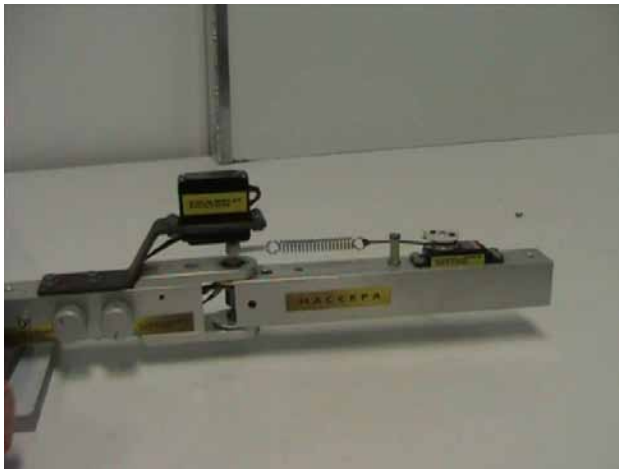
1 motor controls stiffness
